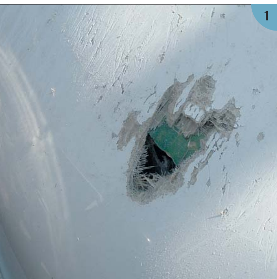
(1) Major damage on a small boat. This dinghy pounded on the rocks for several hours. You can see how a rock punched through the hull and left the gelcoat severely scratched. (2) The damaged area has been cleaned and ground back. A thin piece of plastic-covered plywood has been wrapped around the outside of the hull, and a layer of fiberglass applied from the inside. Note the irregular outline of the hole. Grind only until you reach undamaged laminate. There is no need to grind or cut a smooth perimeter.
