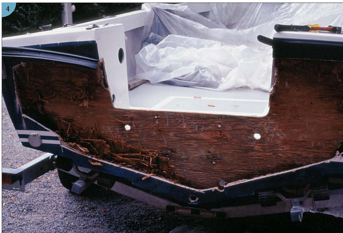
(4) This is what remained of the transom after I removed the rotted core.
