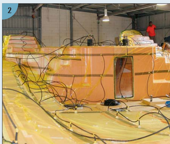
The infusion lines are in place, and as soon as the vacuuming is completed, the valves will be opened and resin will pass through the larger-diameter lines into the laminate. (Courtesy Perry Catamarans, Queensland Composites, and High Modulus)
