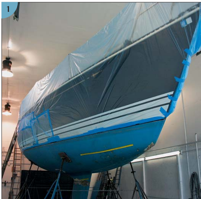
(1, 2, 3) The fiberglass on this boat will be ground back, which will spread fiberglass dust everywhere. To avoid removing all the interior fittings and cushions and having to painstakingly clean the boat after the repair work is done, the workers have taped polyethylene sheeting over all areas not involved in the repair.
