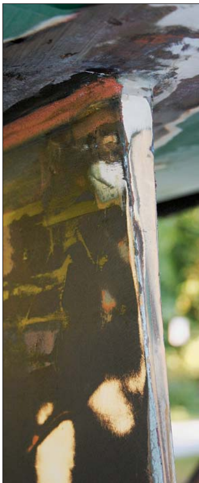
The trailing edge of this keel terminates in a \frac{1}{8} - to \frac{3}{16} -inch (3 to 4 mm) flat, which towing tank testing has shown will actually cause less resistance than a razor-sharp edge. A perfectly sharp trailing edge is extremely hard to achieve in any event, and is also prone to chip or break.
