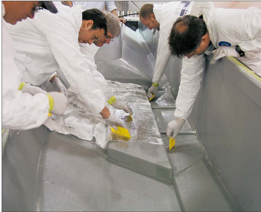
After coating the repair surface with well-mixed resin, lay your fiberglass in the wet resin. Add a little more resin on top of the fiberglass and roll it out to ensure that the entire surface is wet. Work from the center toward the edges to eliminate air bubbles. (Courtesy System Three)
