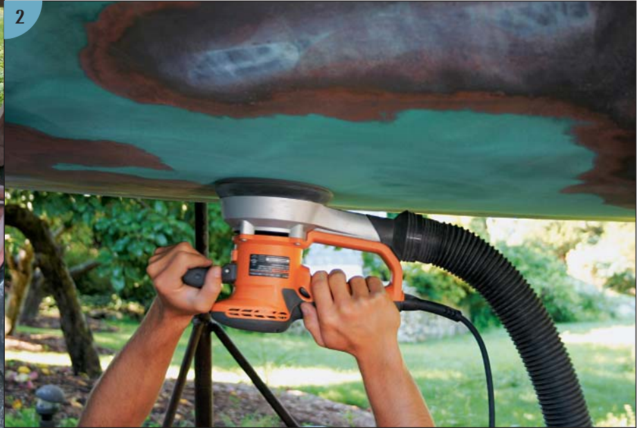
(1) My RIDGID 6-inch random orbit sander attached to the RIDGID shop vac. This method may look a little ungainly, but it keeps the job free of sanding dust and residues. You do, however, need to make sure the holes in the sanding disks align with the holes in the sanding pad. (2) Notice how little dust is generated around the sander in use. Even so, the operator is wearing a respirator and eye and ear protection.
