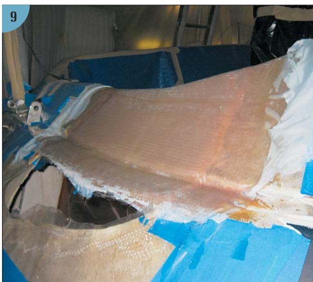
(9) The cutaway portion of the transom had to be laid up again using the same technique as on the hull side, leaving this small hole (between the top of the swept-back transom and the aft rim of the cockpit coaming above it) to be finished.
