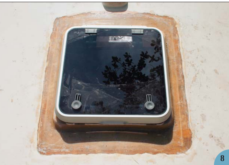
(8) The new hatch sitting on the new boss, ready to be bolted down—which will happen after we've sanded and painted the area around the hatch. At this stage the deck is still slightly flexible, but when the hatch is bolted in place it will help stiffen the deck. It is very important to get the top surface of the hatch boss flat and level. If the boss is not level, it will distort the hatch rim and cause a leak.
