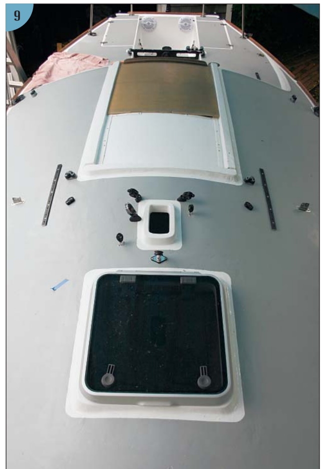
(9) The finished installation after we painted it with Interlux's white Perfection and Interlux's gray Interdeck.
