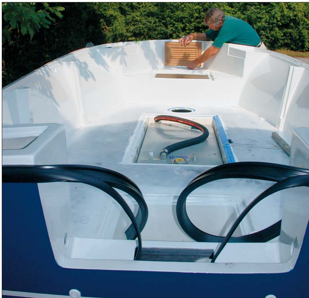
I thought I had finished restoring this 18-foot powerboat, but when I drilled bolt holes in the transom to mount an outboard engine, I found that the transom core was soaking wet. The entire transom had to be replaced. (See Project #4 in Chapter 7.)
