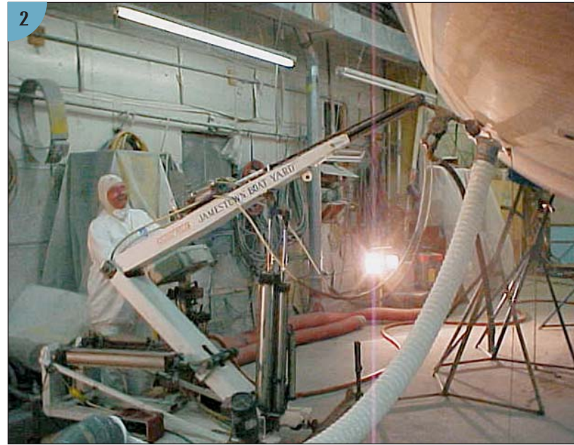
(2) The peeled chips are collected in the tube attached to the peeler head and go directly into the trash.
