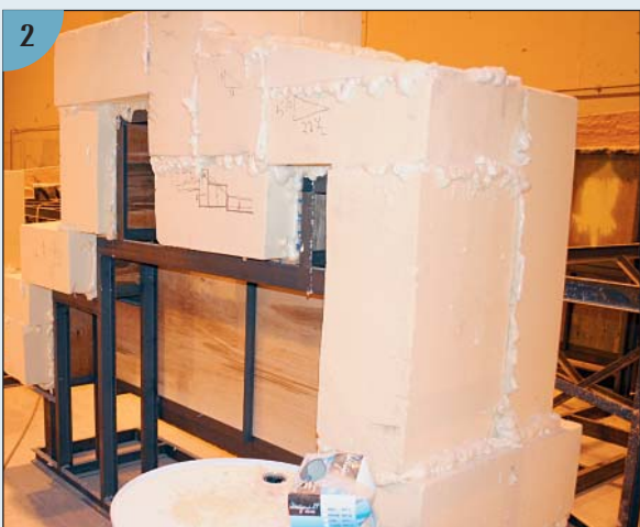
(2) Foam blocks are glued to the armature. Filler foam has been sprayed between the blocks to help glue them together.
