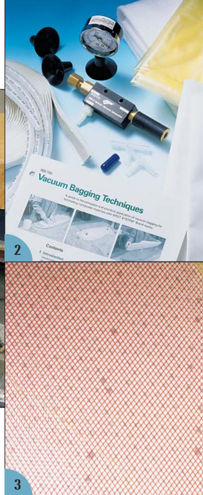
(1) The bow of a yacht under a vacuum bag. (2) This WEST System vacuum-bagging kit contains a venturi vacuum generator, release fabric, bleeder cloth, vacuum membrane, vacuum gauge, tubing, and manual. It costs about $200 (2009). (3) This close-up shows the resin (small dots) coming through the bleeder cloth under the plastic vacuum bag cover.
