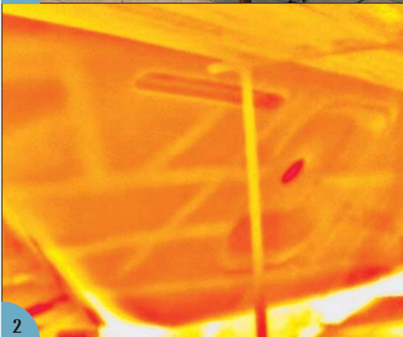
(1) Infrared testing can also be used to find voids in a laminate. Here a hull as seen with the naked eye. (2) The same hull as viewed with an infrared camera. In this case there are no voids present, because no darker patches show up. Note how the hull framing can easily be seen through the laminate using infrared technology. (All infrared images courtesy Mark Ashton, Independent Marine Systems)
