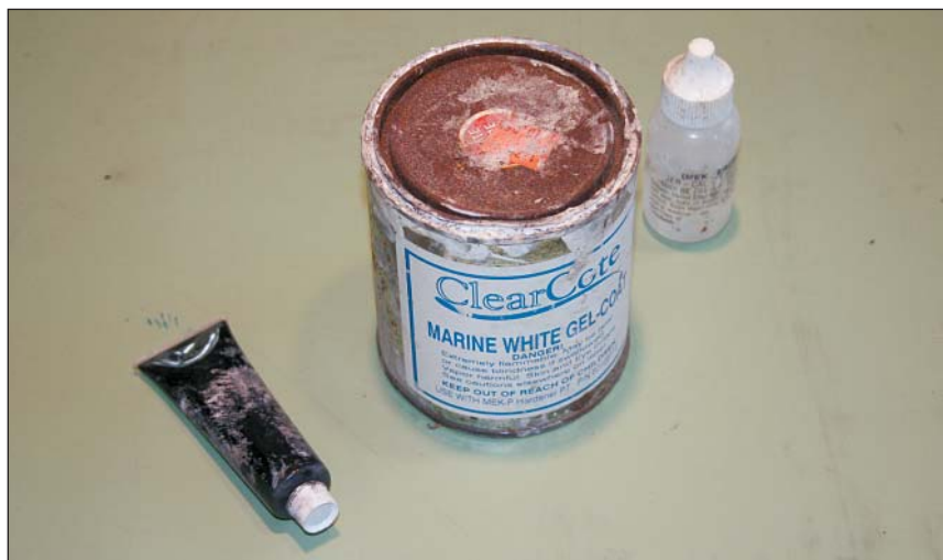
You can purchase small cans of resin (in this case, gelcoat resin) suitable for most small repair jobs at your local chandlery or marine products distributor. Be sure to measure out the resin carefully in order to get a good, strong bond. The bottle to the right rear of this photo contains MEKP, while the tube in the lower left contains a black coloring agent. It only took one or two drips of the black pigment to turn white gelcoat from this can the right shade of gray to repair the 420 shown in Chapter 4.
