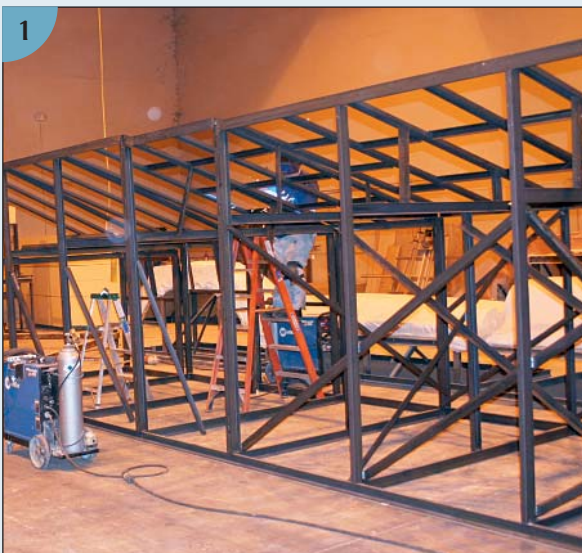
(1) The steel armature for a portion of a large yacht's upperworks is welded together.
