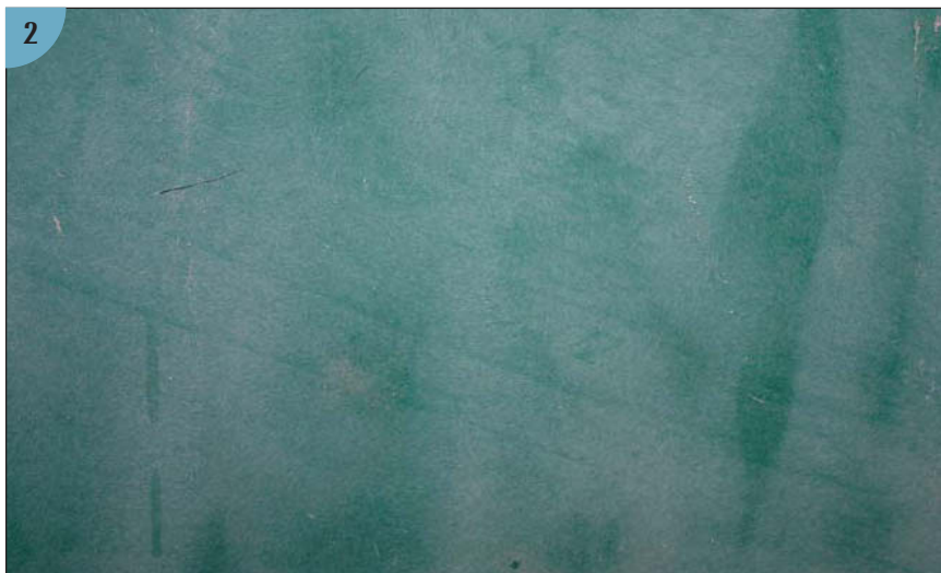
(2) This oxidized gelcoat could have been restored with aggressive compounding, but the hull had sustained other damage and the owner decided to paint the boat. (This is the hull of the J/24 owned by my son; other repairs to this boat are described in Chapters 5 and 7.)
