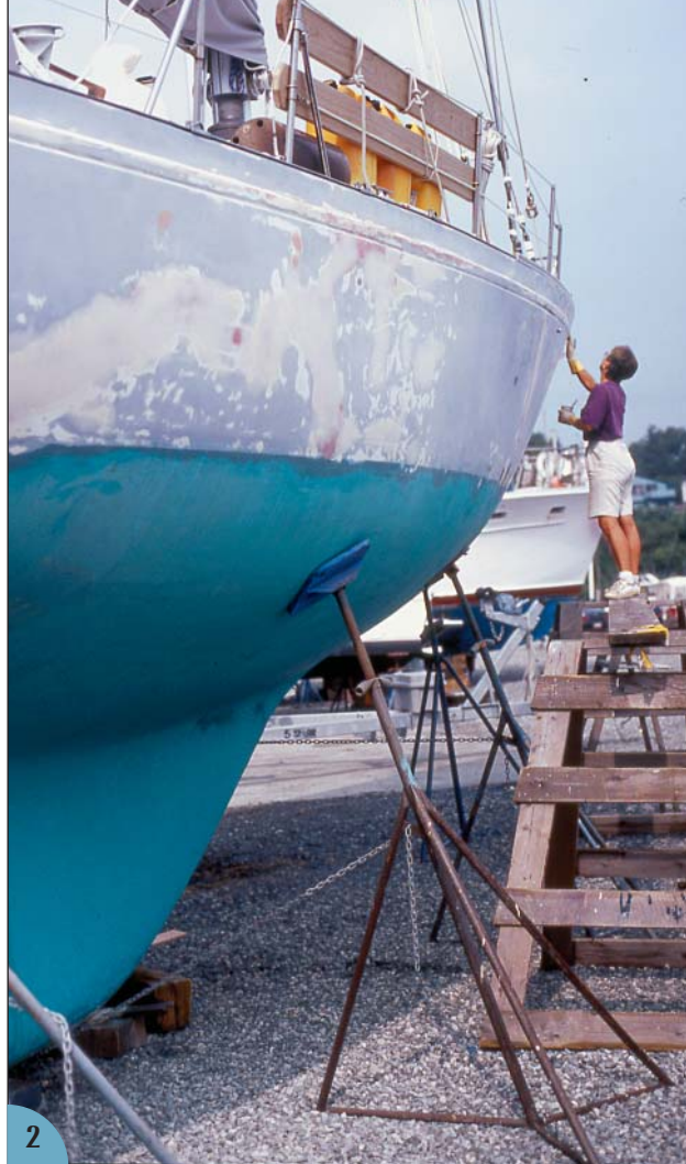
Preparing a hull before painting is critical. This hull is being faired with thickened epoxy prior to sanding and priming (1, 2).
