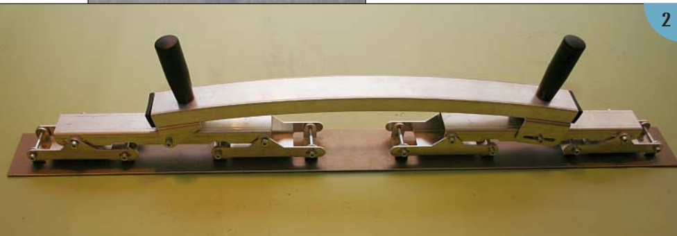
(1) A relatively short longboard that you can purchase from marine stores. The finest grade of sandpaper available for this board is 320-grit, which is about the coarsest grit you would want to use before a final coat of paint. If you'd rather use a finer grit, such as 400, you won't be able to use a longboard of this size. (2) A professional longboard with a flexible blade. This one comes from Flexicat Tools in the Czech Republic; their U.S. website is www.flexicat-usa.com .
