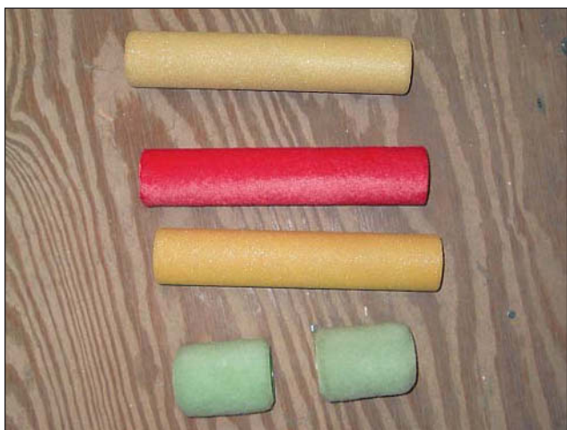
Various rollers used to apply topcoats. The foam rollers shown here are designed for marine paints and will not fall apart. The nylon rollers (pale green) are best used for nonskid.
