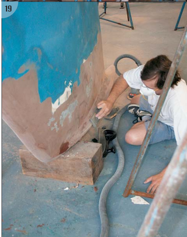
(18, 19) Then they sanded the fairing using a longboard with progressively finer grits. While the hull repair was curing, they turned to the keel, first straightening its tip and then using fairing compound to smooth out the imperfections.
