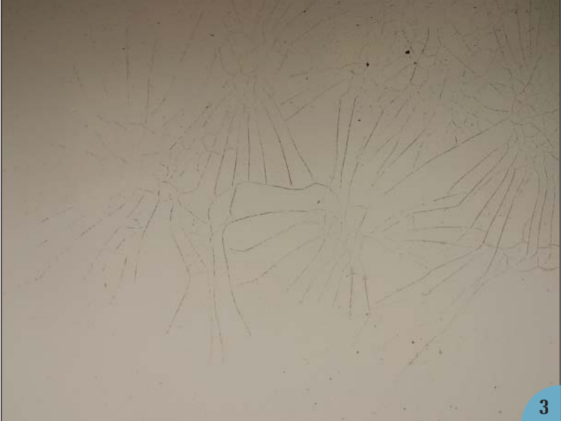
(3) Impact damage on the topside of a single-skin hull. Note the four separate star patterns suggesting four hard impacts, which may have occurred at different times. This damage needs to be fixed as soon as possible so that water cannot penetrate beneath the gelcoat, which can lead to delamination or blistering. If this were a cored hull, you would need to worry about saturation of the core or delamination of the core-to-skin bond.
