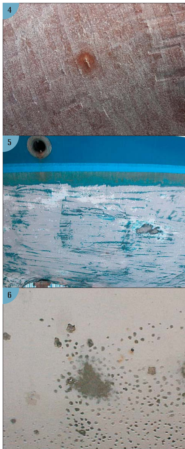
(1) These representative examples of osmotic blistering caused by water penetration into the outer laminate of a hull include blisters after a hull has been peeled, water penetration via blisters into a peeled hull's core (2), which will need to be dried out or replaced, and other examples of blisters (3, 4, 5, 6). (All images courtesy Jamestown Boat Yard.)
