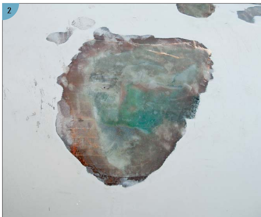
(1) Major damage on a small boat. This dinghy pounded on the rocks for several hours. You can see how a rock punched through the hull and left the gelcoat severely scratched. (2) The damaged area has been cleaned and ground back. A thin piece of plastic-covered plywood has been wrapped around the outside of the hull, and a layer of fiberglass applied from the inside. Note the irregular outline of the hole. Grind only until you reach undamaged laminate. There is no need to grind or cut a smooth perimeter.
