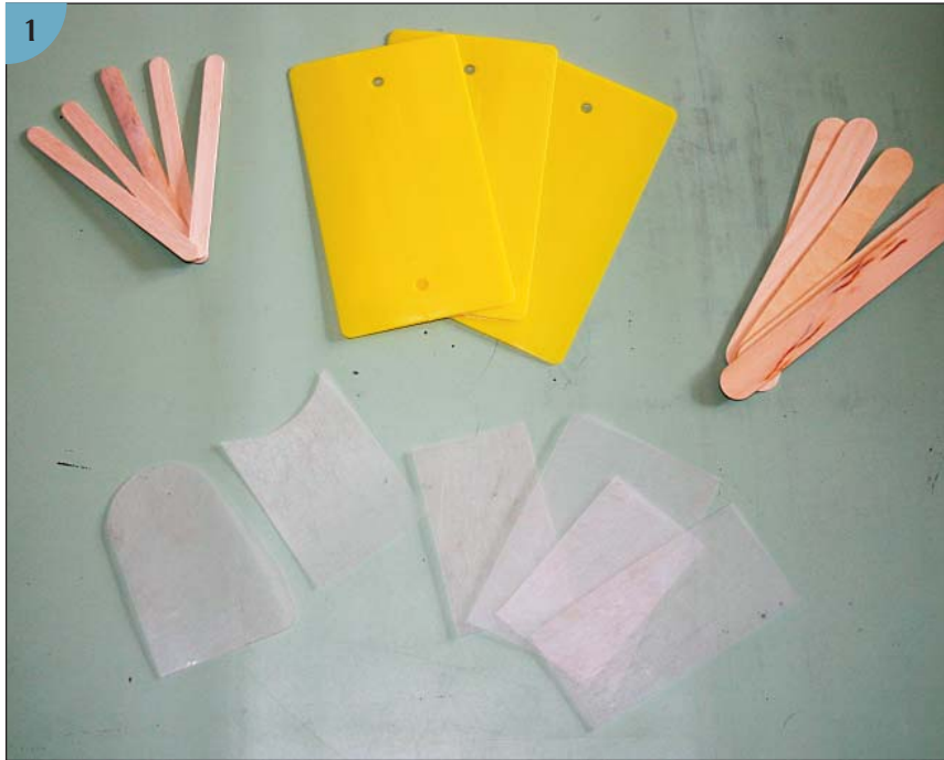
(1) Spreaders and wooden stirring sticks of various sizes are essential for mixing small quantities of resin. I bought the yellow spreaders shown here, but I made the off-white ones from a thin plastic counter mat. You can cut these thin spreaders to any shape and toss them out after using. Clean the spreaders by wiping them with acetone or some other solvent, but check the edge of a spreader after each use. If it becomes nicked, throw it out and use another.
