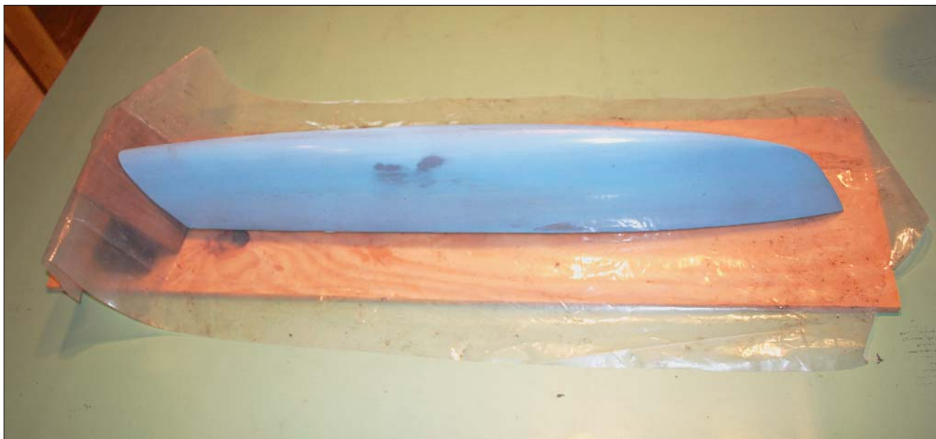
A plug can be made for a model hull, as shown here, just as it can be made for a full-sized hull. This plug has been coated with mold release wax and is sitting on a piece of plastic, ready for the mold laminate to be applied. Any fiberglass part can be molded over a plug like this.
