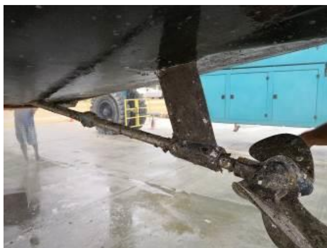
Shaft, strut and prop.
