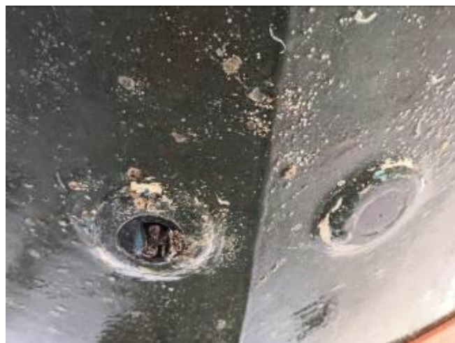
Sounder transducer and speed log.
