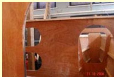
Forward inside view, all inside work is done before the deck is added
