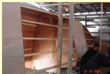
One of the hulls, partly planked
